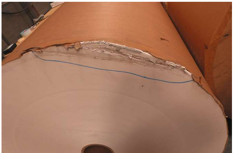
End damage from poor handling. Source: UPM.
