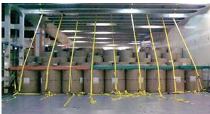
Step-down securing of StoRo cargo. Source: Stota-Enso.
