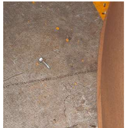
✘ Potential roll end damage source — loose screw. Source: IF P&C.
