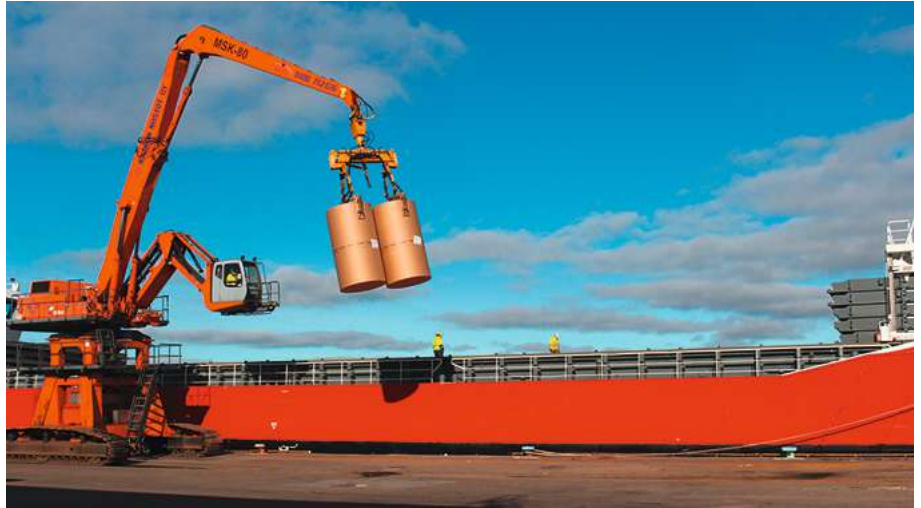
LoLo operation by Mantsinen. A mobile hydraulic crane equipped with clamps for roll loading. Source: Stora Enso.
