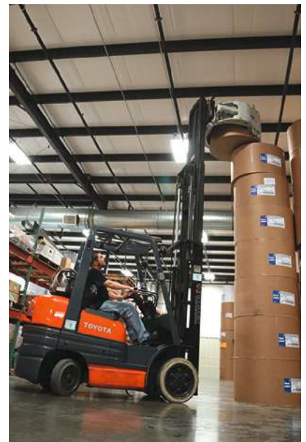
⚠ Paper roll clamps for high stacking should have 0° mounting because a forward tilted mounting has a severe negative effect when stacking. Source: Cascade.
