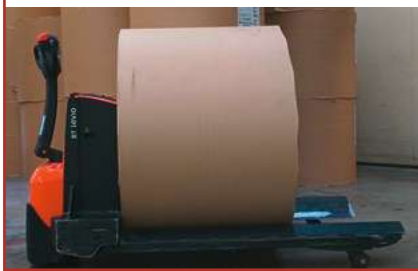
Roll loaded on to an electric truck equipped with angled forks. Source: Mabeg.
