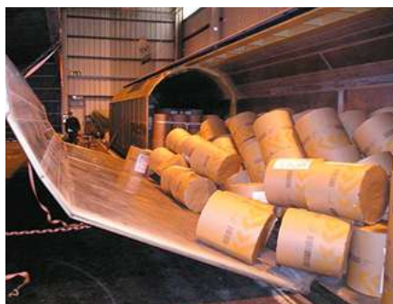
Risk of incorrectly secured loads. Source: IGP.
