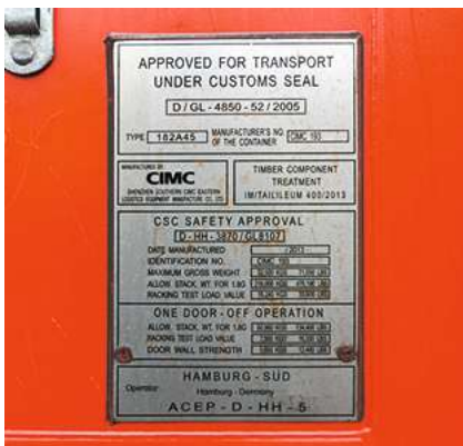
Example of a CSC information plate fixed to container door. Source: INTAKT.
