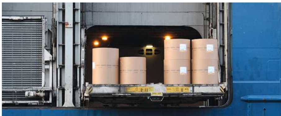
Rolls on sideport conveyor. Source: Stora Enso.
