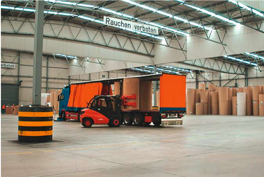
Truck loading inside warehouse, note protection around pillar. Source: 'FMS Use No Hooks'.
