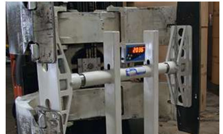
2: A cylinder clamping force indicator uses a hydraulic cylinder to measure the pressure that is then converted by a formula to give the clamping force. Source: Cascade.
