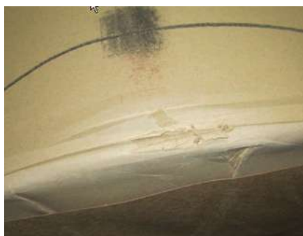
Kissing damage on the bottom edge of the top roll and top edge of bottom roll. Source: Idealliance.
