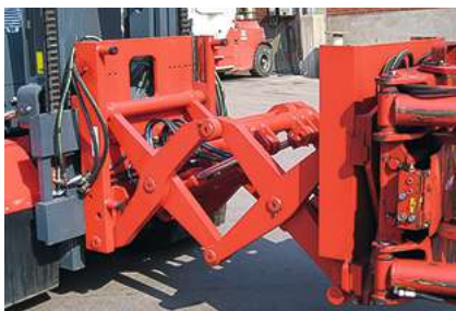
Use clamp extenders when loading standing rolls from one side — rolls must not be pushed. Source: Bolzoni Auramo.
