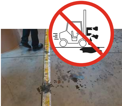
Oil leaks on floor are a high accident risk that need to be cleaned immediately and source repaired. Source: UPM.
