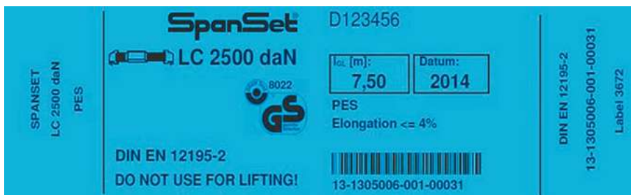
Typical content of webbing strap label, marked in accordance with EN 12195 2. Source: SpanSet/CEPI.
