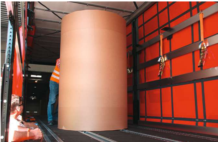
Joloda trailer with rail loading, steel wedges and lashing systems provide optimised securing, transport and handling of paper. Source UPM
