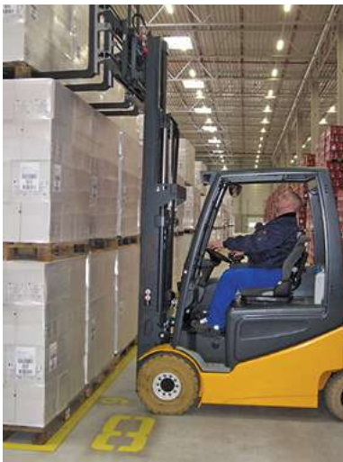
Side-by-side double pallet handler for efficient internal logistics. Source: KAUP.
