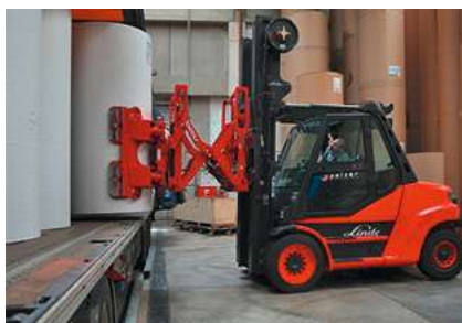
Use clamp extenders when loading standing rolls from one side — rolls must not be pushed. Source: Bolzoni Auramo.
