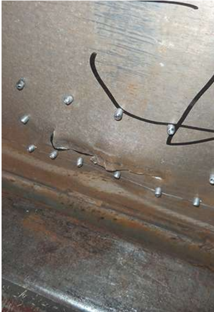
Poor repair of a rail wagon. Source IF P&C
