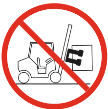
Keep mast vertical when clamping standing rolls
