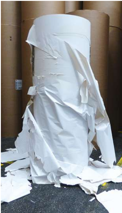
Loose paper from unwrapped part rolls are a fire risk. Always rewrap rolls. Source: UPM.
