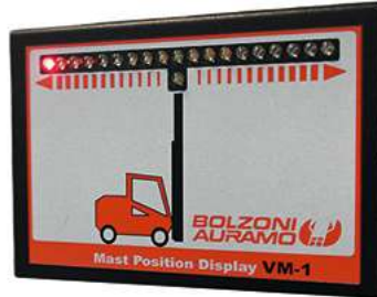
Several types of mast position indicators are available to ensure operators clamp at 0°. Sources: (left) Cascade, (right) Bolzoni Auramo
