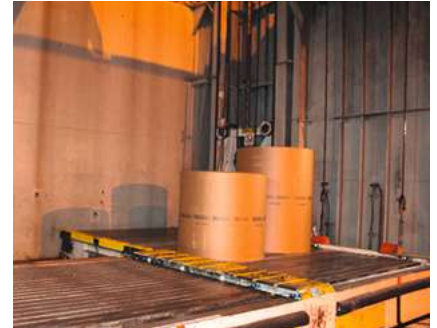
Rolls are moved from elevator to conveyor. Source: Stora Enso.
