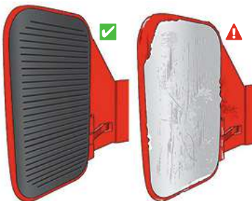
Worn friction surface. Source: Bolzoni Auramo.
