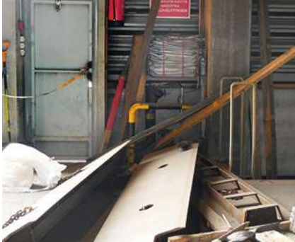
✘ Poor storage practices increase fire risk. Source: IF P&C.
