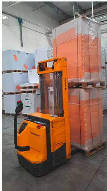
Dual forks used to handle two pallets together. Source: Ecograf.
