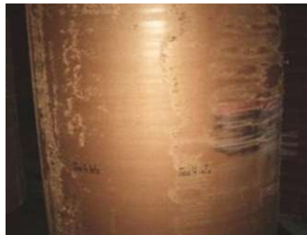
Minor chafe damage is generally caused by vibrations during rail transport Source: Idealliance.
