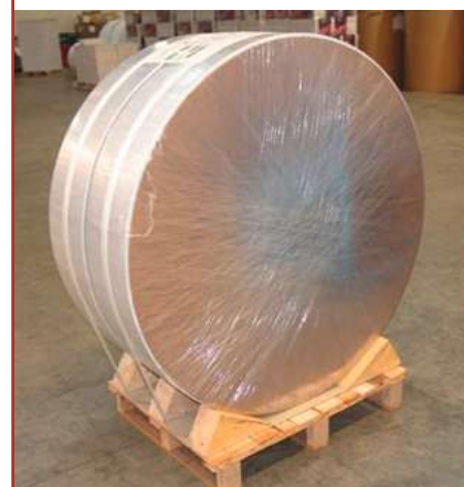
Standing roll loaded on to a pallet and securely chocked both sides. Source: UPM.
