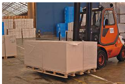
Single-Double used to handle corrugated sheets.
