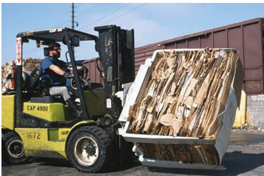
Turnload are often used in recycling operations. Source: Cascade.
