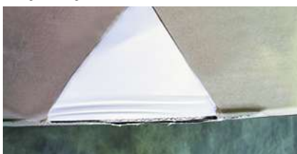
1. Crimped edge damage. Source: Bolzoni Auramo.
