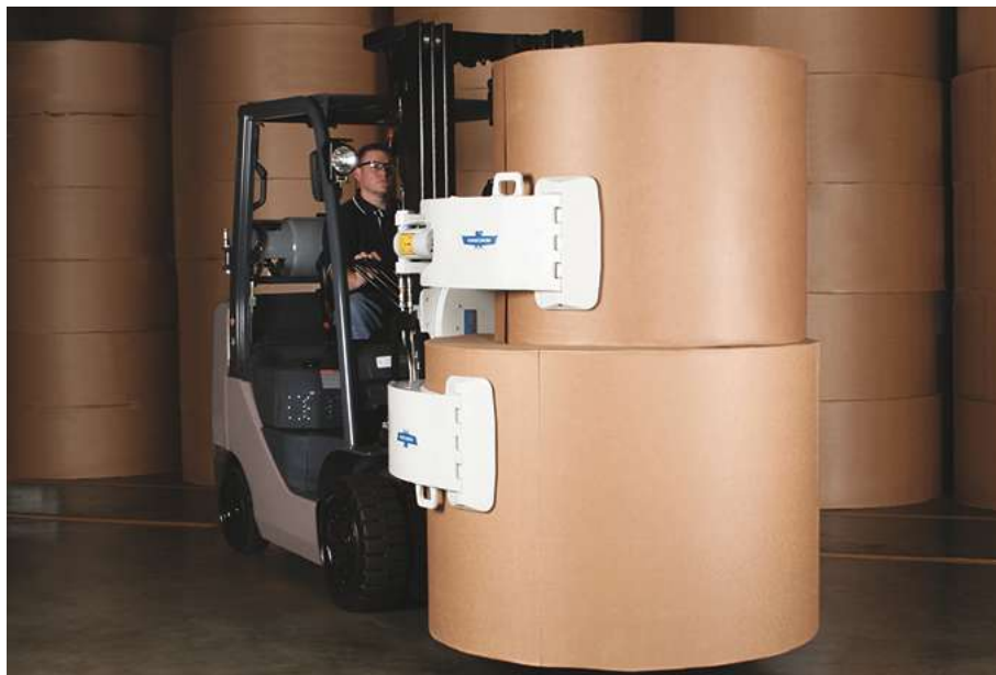
Lift truck equipped for correct handling of two rolls with different diameters. The biggest roll should be on bottom to avoid any risk of roll dropping out. Source: Cascade.
