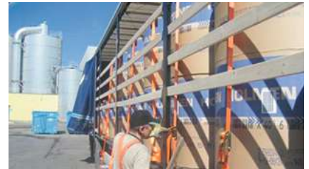
Tighten with ratchet to correct force, (max 50 kg (110 lbs) per ratchet
