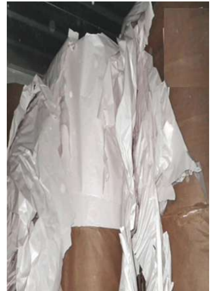
Severe chafe damage from excessive rail transport vibration. Source: Idealliance.
