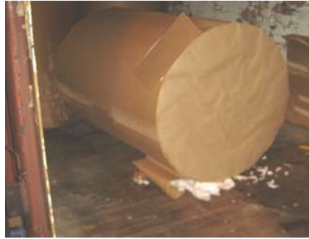
Photographs of toppled rolls help identify rail handling or mill loading errors. Source: Idealliance.
