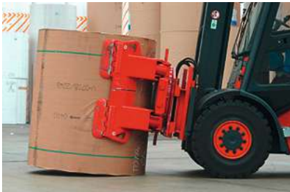
X Avoid off-centre clamping if arms are positioned too far in front of the imaginary centreline of roll. Source: FMS 'Use No Hooks'.
