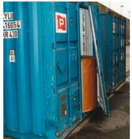
Container door damaged by cargo within. Source: FMS 'Use No Hooks'.
