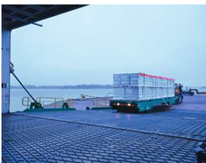
A fully loaded cassette is being pushed into the ship by a Tugmaster. Source: INTAKT.
