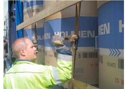
Heavy-duty ratchet for tie-down lashing. Use lashing straps with min. 4000 kg (8818 lbs) breaking strength, pre-tightened 400 kg min-600 kg max. (882-1323 lbs).
