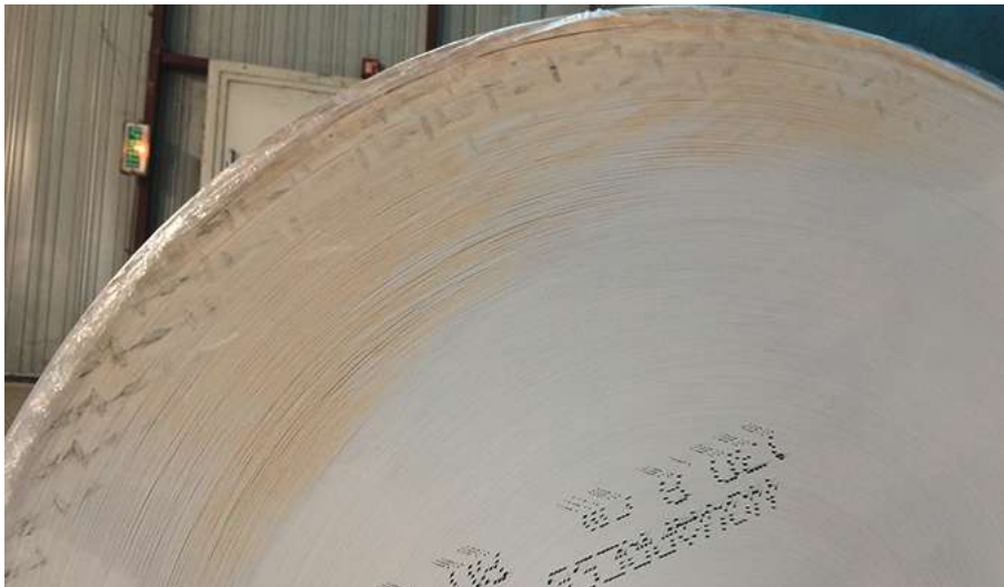
Roll with about 20% water damage. Source: Stora Enso.
