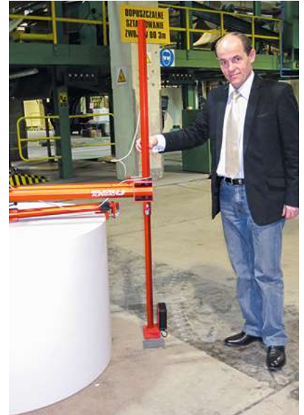
An out-of-round measuring device. Ultrasonic technology can be used to quickly and accurately measure roll roundness without disturbing its wrapping. The results can be viewed on an LCD display and exported to a data management system. Source: Bolzoni Auramo.
