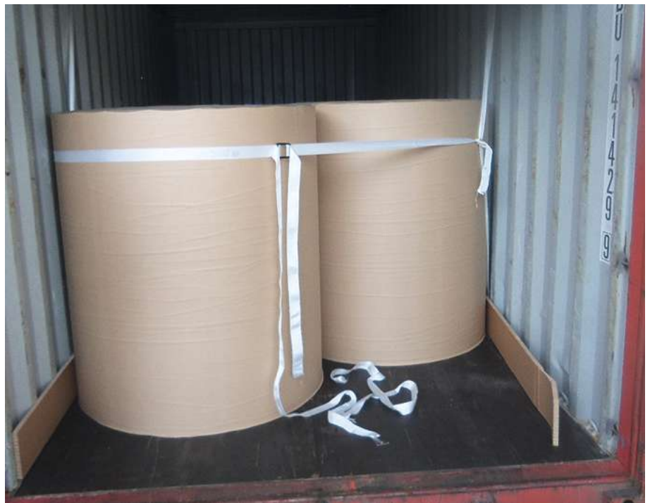
Insufficient blocking. Source: UPM.
