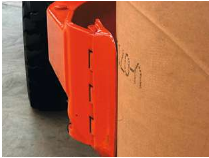
X Clamps insufficiently opened will damage the roll. Source: FMS 'Use No Hooks'.
