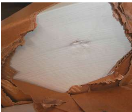
End damaged through wrapper. Source: Stora Enso.
