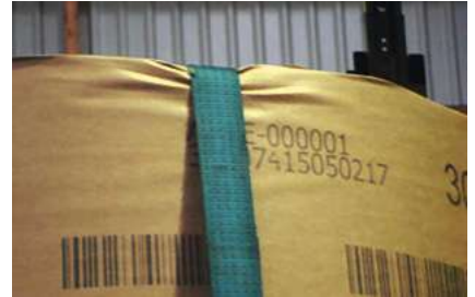
❌ Lack of corner protection will damage cargo. Source: Stora Enso.
