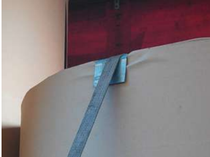
Incorrect edge protection. Source: IF P&C.
