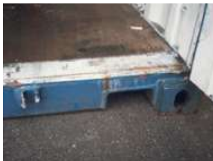
1 Cracked door sill.
