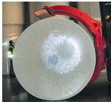
Short arm should be against the floor when lifting a roll from the ground. Source: Bolzoni Auramo.
