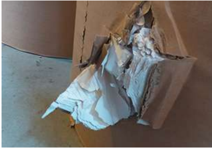
Side damage from poor clamping. Source: UPM.
