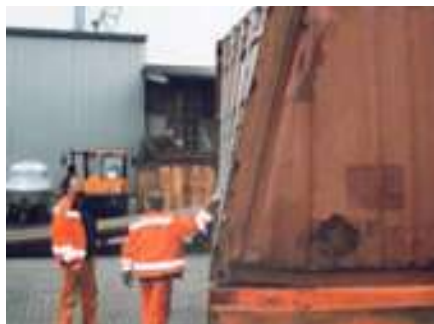
3 Bent door corner post (with j-bar).
