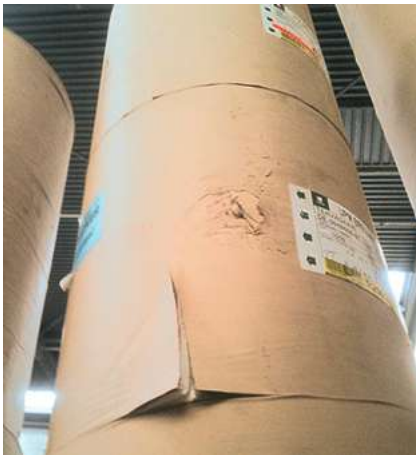
Always repair damage wrapper before stacking. Source: UPM.
