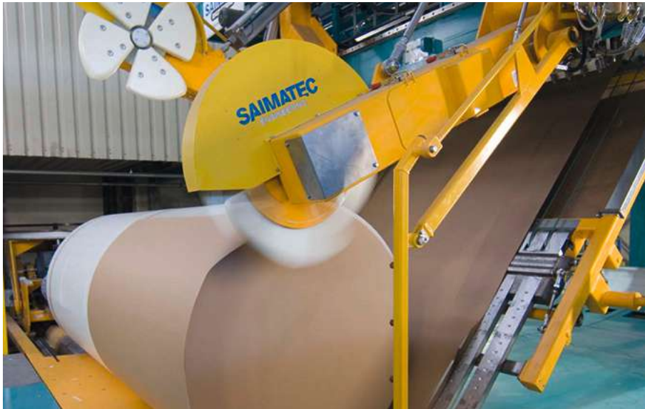
Wrapping operation. Source UPM
