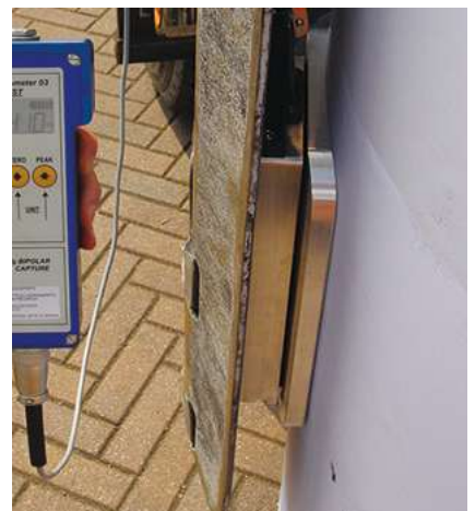
3: Test pad electronic measurement device uses highly accurate weighing cells mounted on a portable aluminium frame. The pad is put between the contact pad and the paper roll and when the clamping arm is closed, the test pad display shows the clamping force. For a split arm clamp, multiply the result with the quantity of split arm sections. This device is suited for quality control supervisors and service staff. Source: Cascade.
