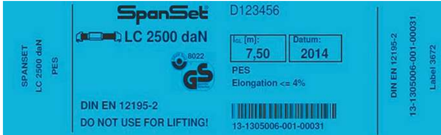
Lashing belts must carry a rectangular, long lasting rating label containing all performance specifications for the lashing. Source: SpanSet
