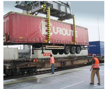
Combi road trailer on rail wagon. Source: INTAKT.
