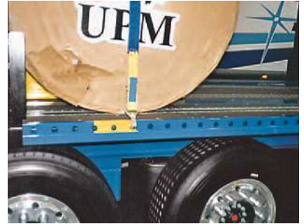
Lashing points on vehicles must conform with either DIN 75410-1 or DIN 12640. If possible, distances between the lashing points should be smaller (= 600 mm / 24 in) than the maximum distance specified in these standards to ensure optimum lashing. Source: SpanSet.
