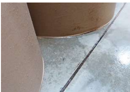
Paper damaged by water leaks. Source: UPM.
