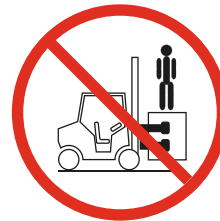
Do not stand on top of the load
