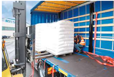
❌ Dangerous position hidden from lift truck driver.
