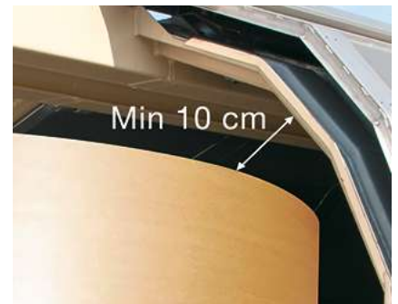
Leave space for rolls that reach the angled part of the sliding doors. Source: INTAKT/OPHAL.
