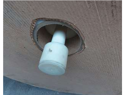
Device used to test core deformation. Source: UPM.
