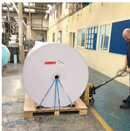
Lying roll loaded on a pallet, where it is securely chocked and strapped down. Source: Stora Enso.
