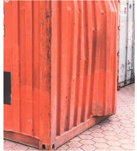
Container wall damaged by the cargo within. Source: FMS 'Use No Hooks'.
