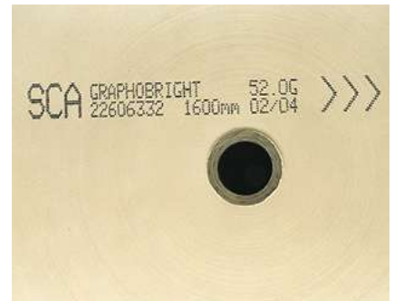
Ink jet printing on roll end shows roll number, weight, unwind direction and mill splice position. Source: WOCG/icmPrint.
