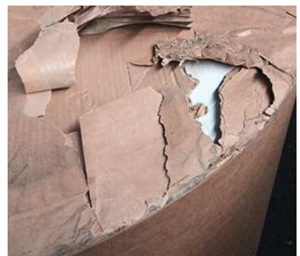
Reel end damage top. Source: Stora Enso.
