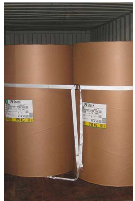
Rolls secured with a horizontal belt with its buckle placed between the rolls. Source: UPM.
