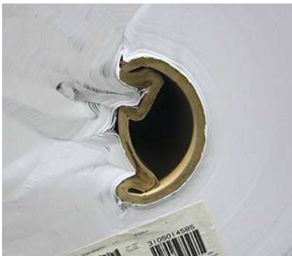
Core damaged beyond repair. Source: UPM.
