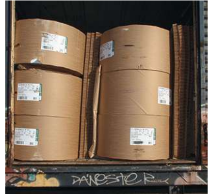
Dunnage used between rolls to reduce shifting of standing rolls. Source: INTAKT.
