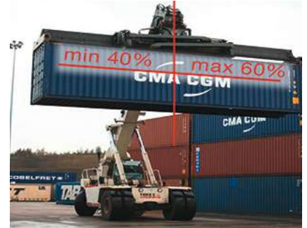
A container load must be balanced correctly to avoid handling difficulties, accidents, and load instability on a carrier. A rule of thumb is to ensure that cargo weight is distributed within a 60-40 % ratio around the centre of the container. Source: Holmen.
