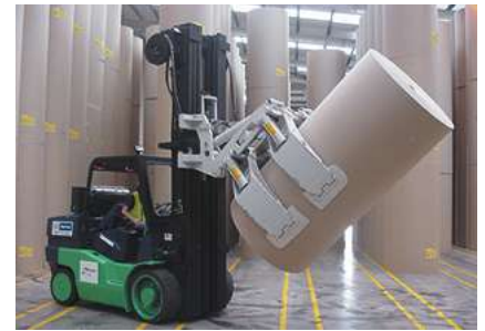
Roll upender clamp tilts the roll forward from vertical to horizontal position to load vehicles from one side. Clamping the roll close to the bottom avoids it hitting the mast when upending or rotating. Source: Cascade.
