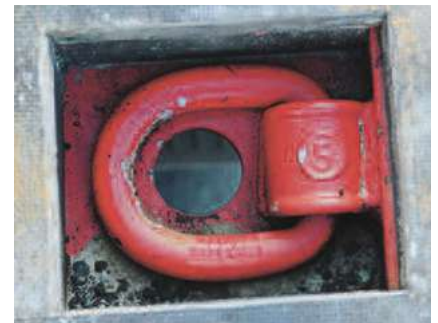
Heavy duty lashing point with load capability of 5 tonnes (11 023 lbs) for lifting and possibly 10 tonne for load securing. Source: SpanSet.
