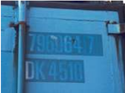
10 Data sign board unsatisfactory and/or missing (CSC/Customs/TCT/Owner & manufacturer's plates).
