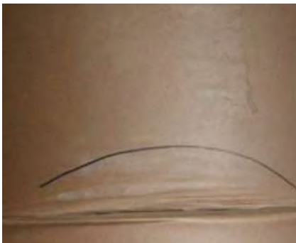
A transit wrinkle can occur even with wall dunnage. This "wear strip" is caused by the wall dunnage that protected this roll otherwise there would be paint on the roll. Source: Idealliance.
