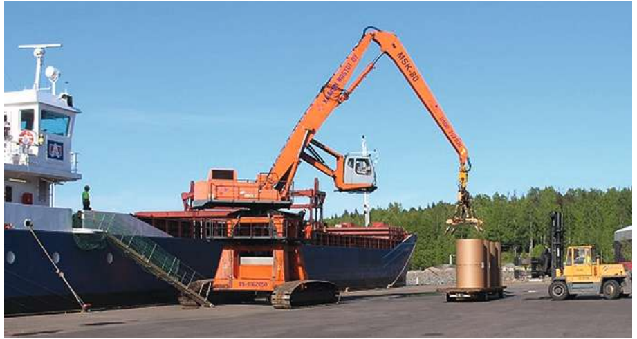
Mobile hydraulic harbour crane loading a LoLo vessel. Source: Stora Enso.
