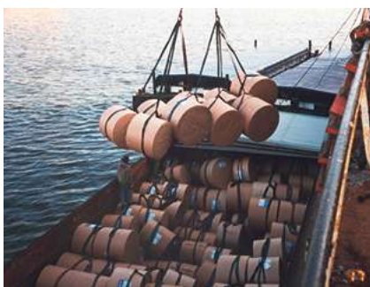
Poor stowage in general cargo vessel. Source: FMS 'Use No Hooks'.
