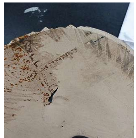
Roll damage from a wet and rusty vessel floor. Source: UPM.
