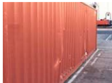
20 Dented external side panel.
