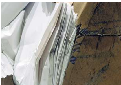
Edge damage. Source: WOCG/icmPrint.
