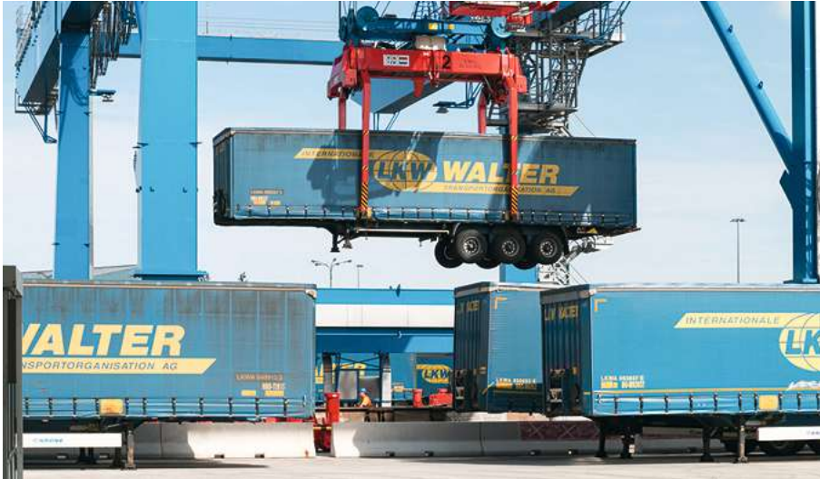
Road trailers are also used in multi mode transport on trains and ships. Source: LKW Walter.
