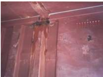
12 Holed internal side panel.
