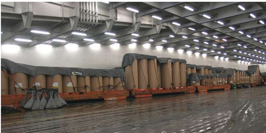
Cassettes must be firmly secured to the deck to resist the forces from all of the vessel's movements. Source: INTAKT.
