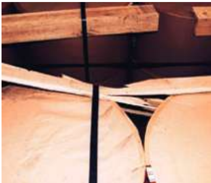
Strips of wood as edge protectors. Source: FMS 'Use No Hooks'.
