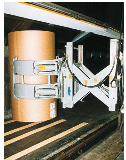
Clamps can be equipped with load extenders to facilitate loading. Source: Cascade.
