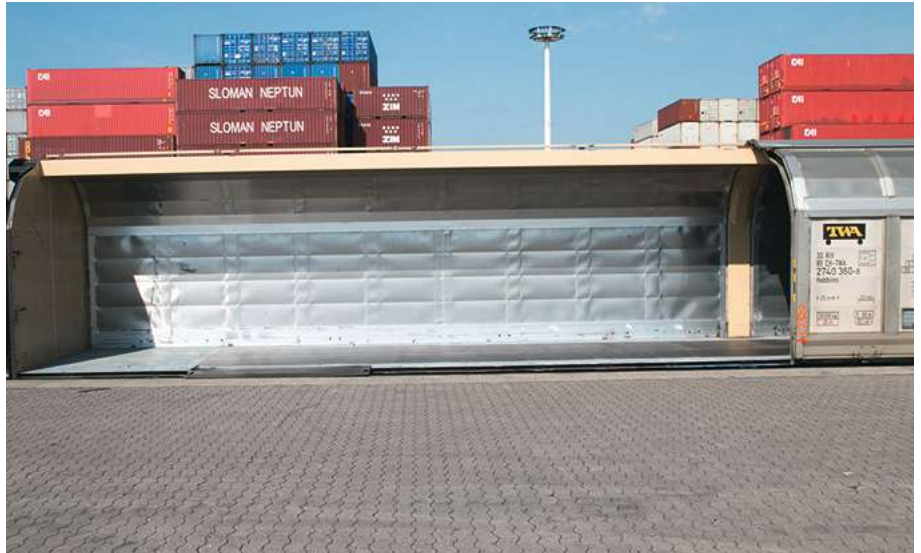
Heavy duty sliding wall commonly used in Europe. Source: INTAKT.
