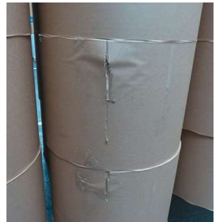
Damage due to sharp clamp pad edge. Source: UPM.
