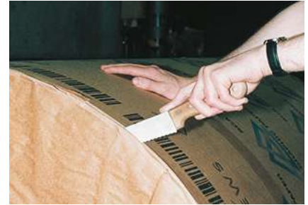
Remove end covers with a broad-bladed knife. Source: WOCG/icmPrint.
