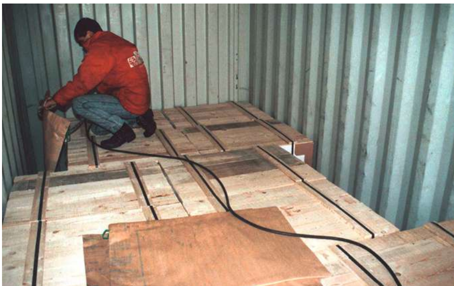
Securing with airbags. Source: FMS 'Use No Hooks'.
