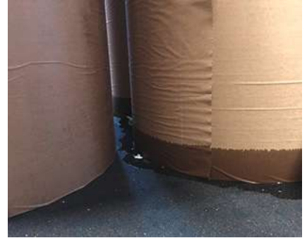
Water damaged roll. Source: Stora Enso
