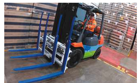
Fork positioners are the most suitable solution to handle pallets of sheet paper because they can be adapted easily to different pallet sizes. Source: KAUP.
