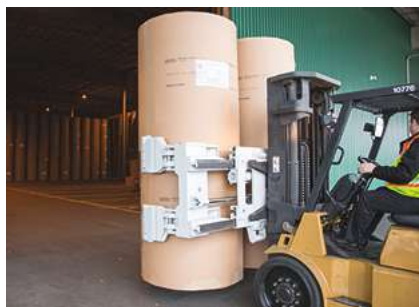
Sliding arm paper roll clamp without a centre arm. Source: Cascade.
