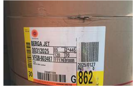
Edge damage due to wrong strapping. Source: Stora Enso.
