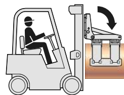
Tilt roll forward. Caution: verify the centre of gravity for the load does not exceed the capacity of the truck. Consult OEM as required.
