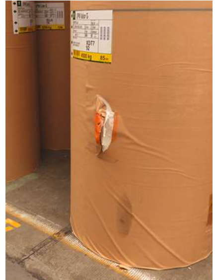
Side damage (belly) caused by a clamp truck's counter weight. Source: UPM.
