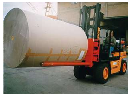
Horizontal paper rolls can also be handled with tine clamps. Source: Bolzoni Auramo.
