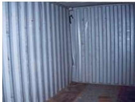
13 Dented internal front panel.
