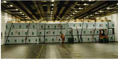
Securing of timber packages with lashing belts. Source: IF P&C.
