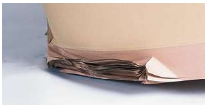
1. Edge damage. Source: Cascade.
