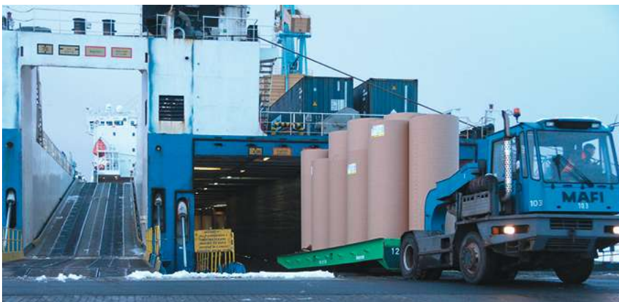
Rolls on a cassette being towed off the ship by a MAFI tractor. Source INTAKT.
