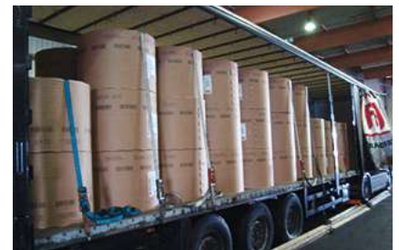
Use straps and edge protectors to secure the rolls. Source: Stora Enso.
