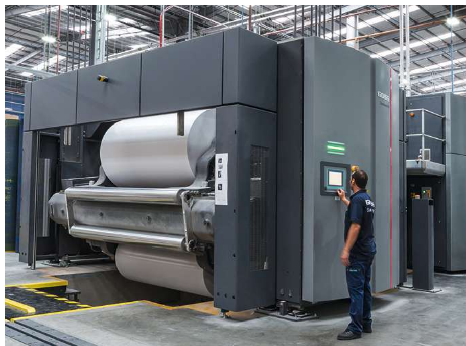
Flying splicer pastes at full production speed. Source: Goss.
