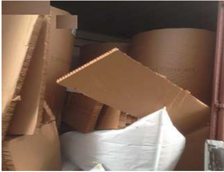
Excessive wagon handling can result in significant damage. Source: Idealliance.
