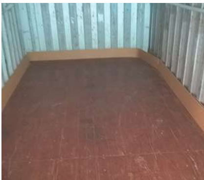
Plywood or corrugated cardboard is placed as protection around the sides and in front of the door. Source: UPM.
