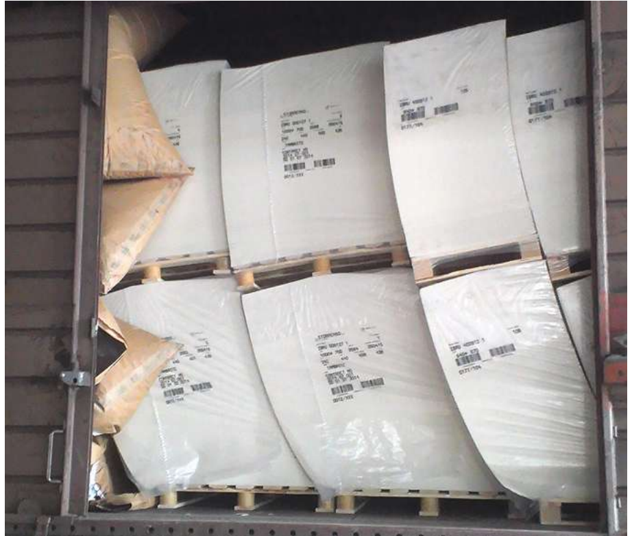
Pallets that have shifted during rail transport. Source: Stora Enso.
