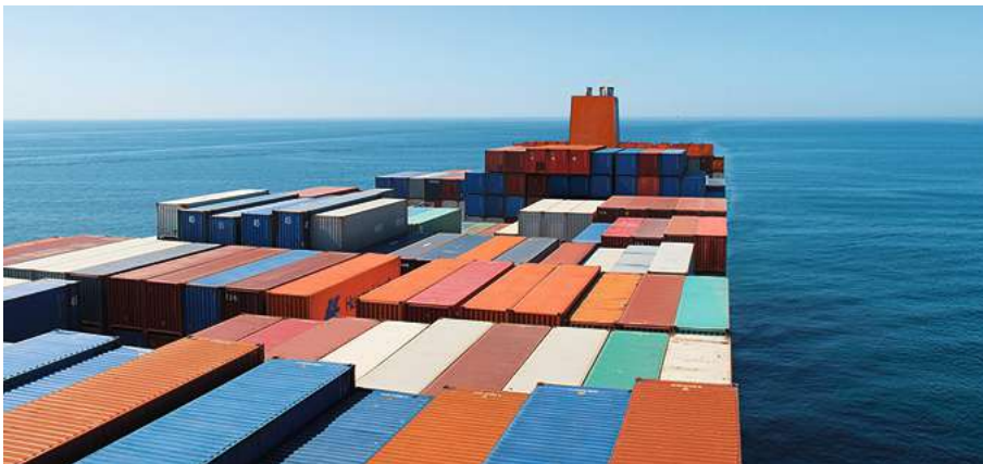
Containers exposed to the sun can have temperature variations of 20-30°C (68-86°F). Any moisture trapped inside will evaporate and when the temperature falls at night condenses and drops onto the paper cargo. Source: Hapag-Lloyd.
