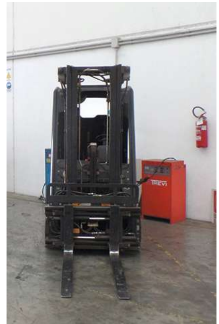
Charging station for lift trucks. Source Ecograf.
