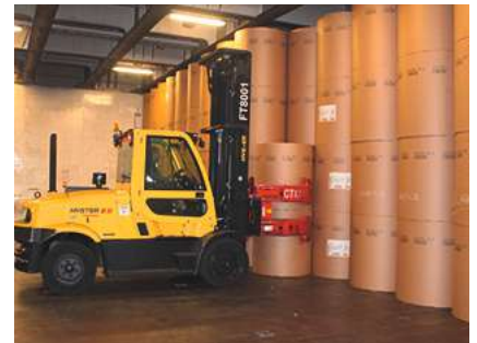
Precise final roll stowing in StoRo hold. Source: Stora Enso.
