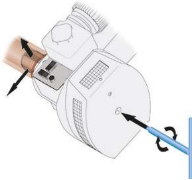
Ensure chucks are fully retracted and free of debris before loading and roll brake is switched on. Source: WOCG/icmPrint.
