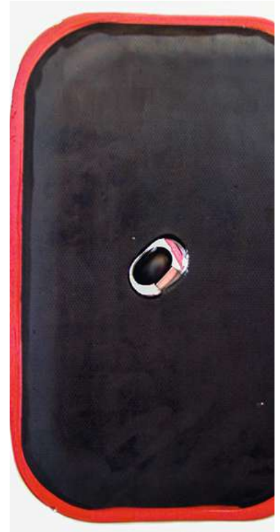
Electronic slip sensors are mounted on the long arm contact pads to measure the paper roll movement in relation to the contact pads. Source: Bolzoni-Auramo.
