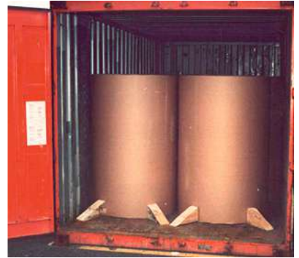
Insufficient blocking / bracing. Source: FMS 'Use No Hooks'.
