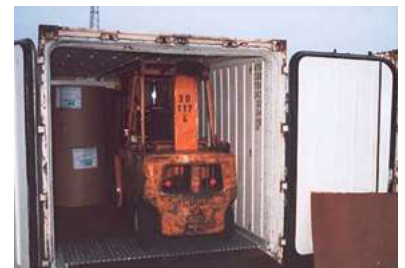
Containers impose height and weight limits on lift trucks.
