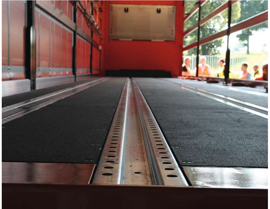
Rails in a Joloda trailer optimise securing and transport of paper rolls. Source: UPM.
