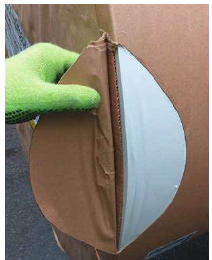
Example of roll edge damage from lack of protection. Source UPM
