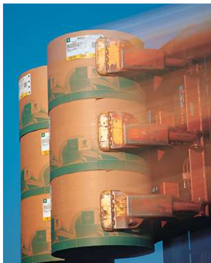
Multiple rolls of graphic paper can be moved with multi clamp trucks. Source: UPM.
