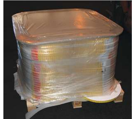
Slipped cargo unit. Photo FMS.
