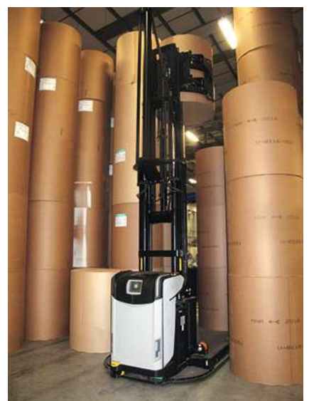
AGV automated roll handling. Source: KBA.
