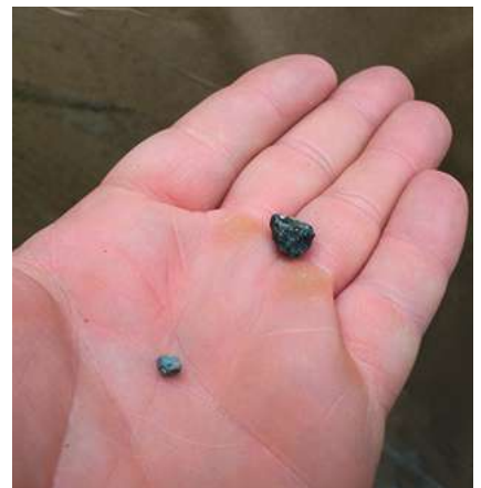
✘ Potential roll end damage source — gravel. Source: UPM.
