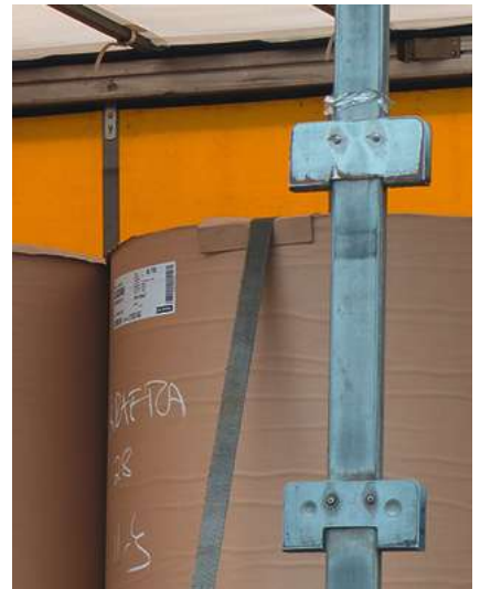
❌ Poor corner protection will damage cargo. Source: Stora Enso.
