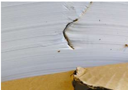
End damage from debris in floor. Source: WOCG/icmPrint.
