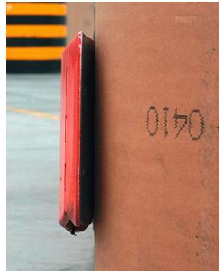
Gap between contact plate and roll. Possibly caused by incorrect position of clamp arms or too small clamp arms. Source: FMS 'Use No Hooks'.
