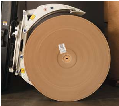
A 5° forward tilt ensures that the short arm pad is under the paper roll and the long arm pad is over the top. Source: Cascade.
