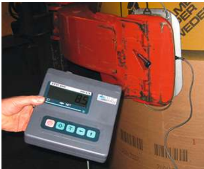
Check the clamping force is correct. Upper Source: Cascade. Lower Source Bolzoni Auramo.
