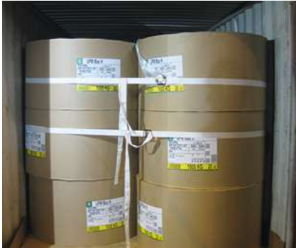
Cargo is secured with horizontal belts. The three tiers of rolls are secured with two belts, around the second and third tiers. Source UPM
