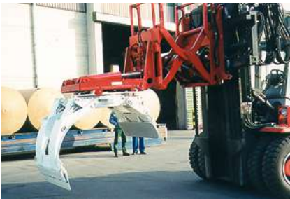
Lifting capacity reduces when the load centre moves forward, for example when using a load extender. Source: Bolzoni Auramo.
